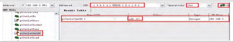
If OID: p1OutletOnOff of socket is chosen, according to the above reading methods, switch state of this socket is read, result of read is closed: "off (0)".
