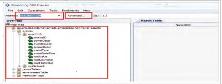
Input PDU IP address (In this case, it is: 192.168.0.254), and input it to address box. Then click "Advanced..."Button to enter the connection Settings.
