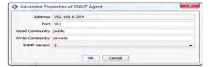
Choose 1 for "SNMP Version", set connection parameters of SNMP v1. In the same way, Choose 2, set connection parameters of SNMP v2. The following default community is set according to factory settings:
