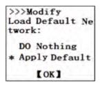
"Apply Default" is loaded with Factory Settings; Restore factory IP, user and password.
