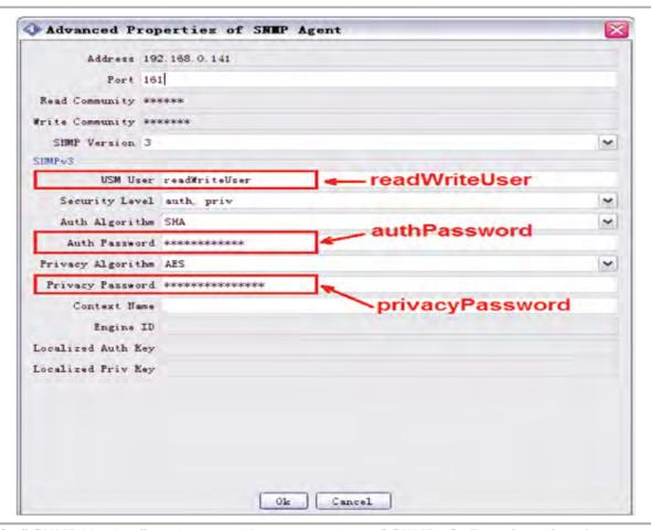
Choose 3 for SNMP Version, set connection parameters of SNMP v3. Based on the above figure ,parameters are set: users, security levels, encryption method, password. As for user, readWriteUser default passwords are as follows:
